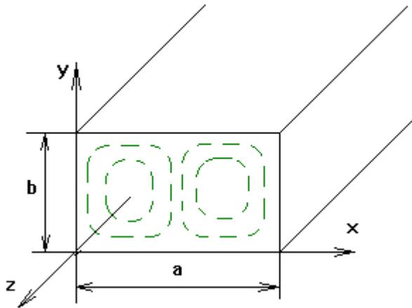
ОТВЕТЫ: 1.  $\{H_y^{E21} \sim \cos^{2\pi x/a} \sin^{\pi y/b}\}$ . 2.  $\{H_y^{E12} \sim \cos^{2\pi x/a} \sin^{\pi y/b}\}$ . 3.  $\{H_y^{H12} \sim \cos^{2\pi x/a} \sin^{\pi y/b}\}$ . 4.  $\{H_y^{H21} \sim \cos^{2\pi x/a} \sin^{\pi y/b}\}$ . 5.  $\{H_y^{E21} \sim \cos^{2\pi x/a} \cos^{\pi y/b}\}$ .
