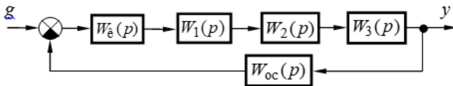
$$W_1(p) = \frac{k_1}{T_1 p + 1}, W_2(p) = k_2, W_3(p) = \frac{k_3}{p}, W_{oc}(p) = k_{oc}, k_1 = 2, k_2 = 5, k_3 = 10 \text{ с}^{-1},$$
