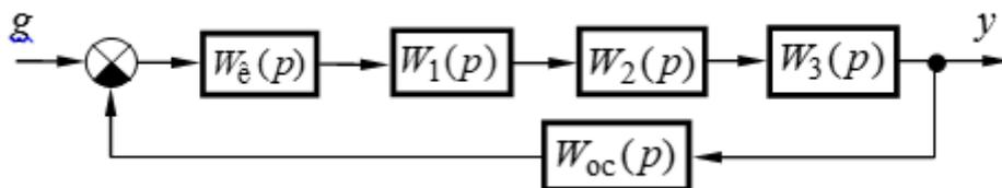
$$W_1(p) = \frac{k_1}{T_1 p + 1}, W_2(p) = \frac{k_2}{T_2 p + 1}, W_3(p) = k_3, W_{oc}(p) = k_{oc}, k_1 = 10, k_2 = 2, k_3 = 3, \\ k_{oc} = 0.5, T_1 = 0.05 \text{ с}, T_2 = 0.03 \text{ с}.$$
