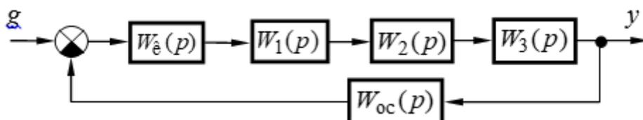
$$W_1(p) = \frac{k_1}{T_1 p + 1}, W_2(p) = \frac{k_2}{T_2 p + 1}, W_3(p) = k_3, W_{oc}(p) = \frac{k_{oc}}{T_{oc} p + 1}, k_1 = 2, k_2 = 5,$$
