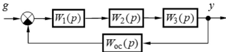
$$W_1(p) = \frac{k_1(\tau_1 p + 1)}{p}, W_2(p) = \frac{k_2}{T_2^2 p^2 + 2\xi T_2 p + 1}, W_3(p) = k_3, W_{oc}(p) = k_{oc}; k_1 = 4 \text{ с}^{-1},$$
