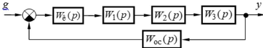
$$W_1(p) = \frac{k_1(\tau_1 p + 1)}{p}, W_2(p) = \frac{k_2}{T_2 p + 1}, W_3(p) = \frac{k_3}{T_3 p + 1}, W_{oc}(p) = k_{oc}, k_1 = 10 \text{ с}^{-1},$$
