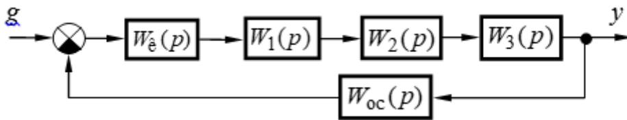
$$W_1(p) = \frac{k_1}{p}, W_2(p) = \frac{k_2}{T_2 p + 1}, W_3(p) = \frac{k_3}{T_3 p + 1}, W_{oc}(p) = k_{oc}, k_1 = 10, k_2 = 2, \\ k_3 = 3, k_{oc} = 0.5, T_2 = 0.01 \text{ с}, T_3 = 0.4 \text{ с}.$$
