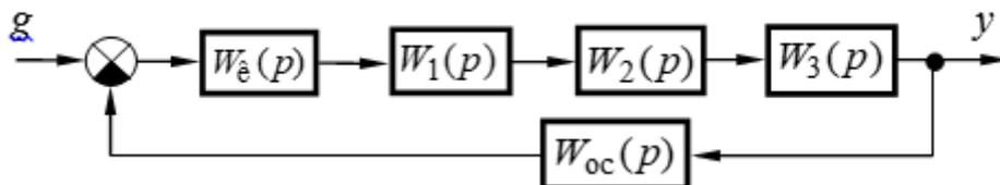
$$W_1(p) = \frac{k_1}{p}, W_2(p) = \frac{k_2}{T_2 p + 1}, W_3(p) = k_3, W_{oc}(p) = k_{oc}, k_1 = 10 \text{ с}^{-1}, k_2 = 2, k_3 = 3,$$
