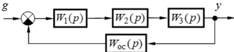
$$W_1(p) = \frac{k_1}{T_1 p + 1}, W_2(p) = \frac{k_2}{T_2 p + 1}, W_3(p) = \frac{k_3(\tau_3 p + 1)}{T_3 p + 1}, W_{oc}(p) = k_{oc}; k_1 = 3, k_2 = 2, k_3 = 5, k_{oc} = 0.8, T_1 = 0.75, T_3 = 0.15, T_2 = 0.3, \tau_1 = 0.03$$
