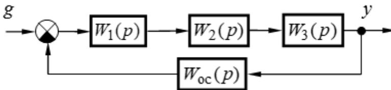
$$W_1(p) = \frac{k_1(\tau_1 p + 1)}{p}, W_2(p) = \frac{k_2}{T_2 p + 1}, W_3(p) = \frac{k_3}{T_3 p + 1}, W_{oc}(p) = k_{oc}; k_1 = 5 \text{ с}^{-1}, k_2 = 2,$$
