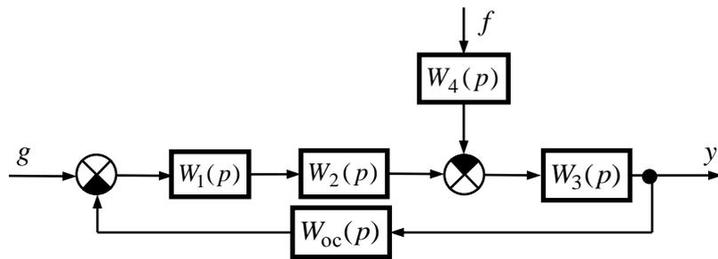
$$W_1(p) = \frac{k_1}{T_1 p + 1}, \quad W_2(p) = \frac{k_2(\tau_2 p + 1)}{T_2 p + 1}, \quad W_3(p) = \frac{k_3(\tau_3 p + 1)}{T_3^2 p^2 + 2\xi T_3 p + 1}, \quad W_4(p) = k_4, \quad W_{oc}(p) = \frac{k_{oc}}{T_{oc} p + 1};$$
