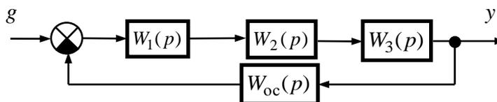
$$W_1(p) = \frac{k_1(\tau_1 p + 1)}{p}, W_2(p) = \frac{k_2}{T_2 p + 1}, W_3(p) = \frac{k_3}{T_3 p + 1}, W_{oc}(p) = k_{oc};$$
